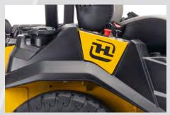
**DUAL ROTO-MOLDED FUEL TANKS**8.5 gallon fuel capacity and dual fuel gauges.
